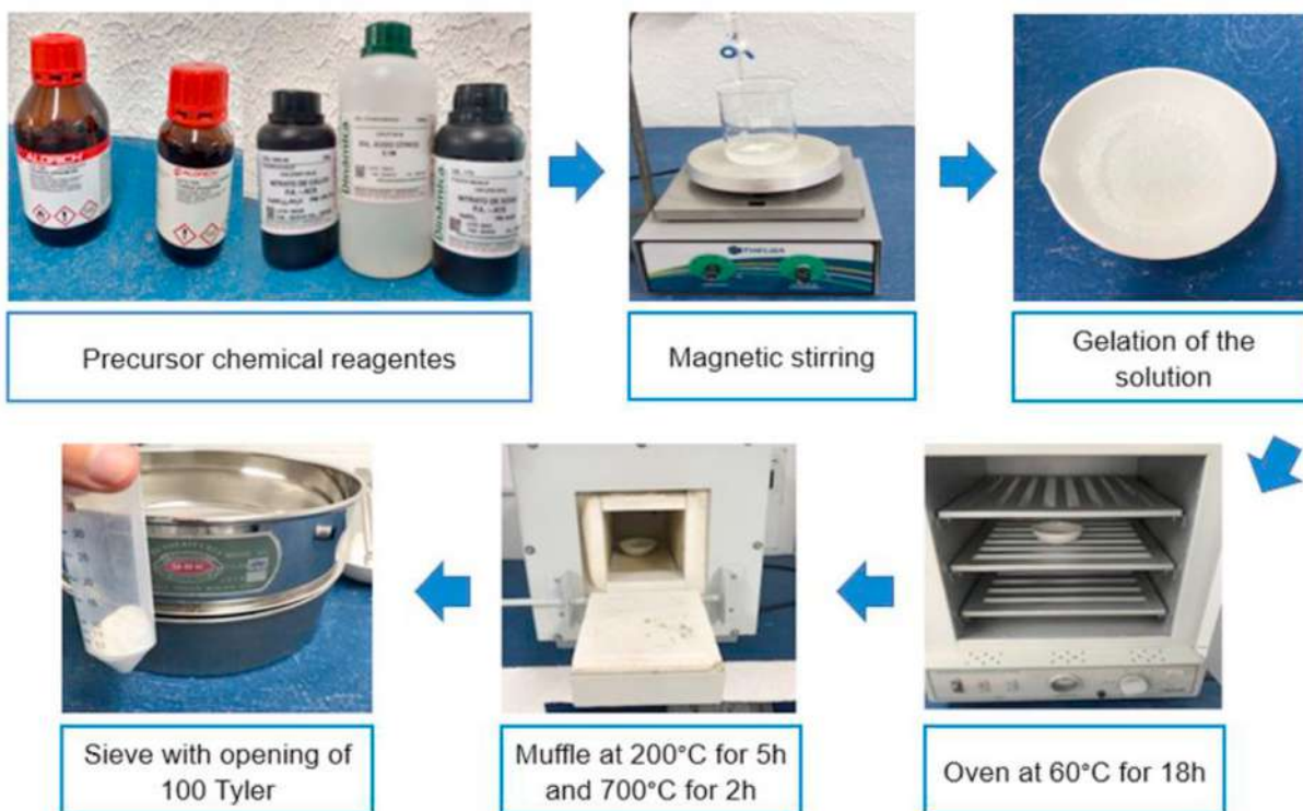
Fig. 1 – Schematic diagram of bioglass synthesis by the sol-gel method.
